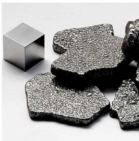
Left: iron in two forms — a machined cube and rough pieces of the raw metal. Right: the body-centred cubic cell, iron's arrangement at room temperature: one atom at each corner of a cube and one more at its centre.
